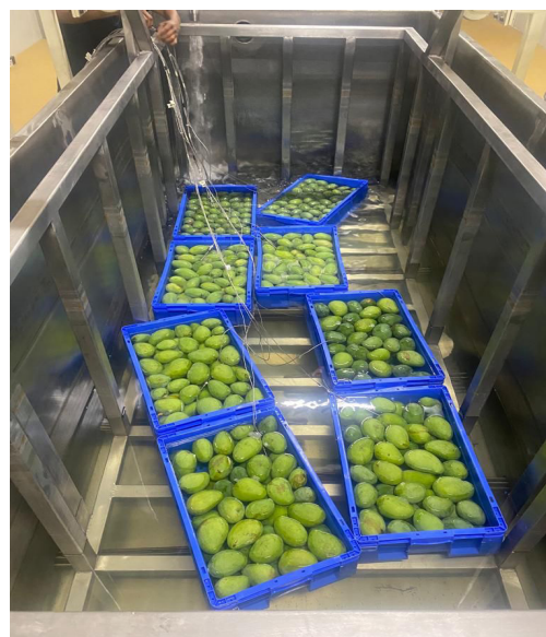
Fig. 3: Thermal disinfection immersion treatment process at a registered facility
